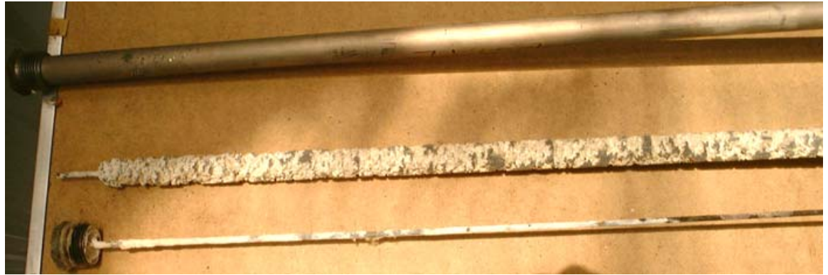
Anode rod at new, partially depleted, and completely depleted stage.
