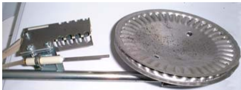
Burner assembly showing correct flame rod positioning
