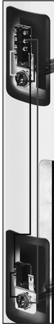
Figure 4 - Therm-O-Disc Thermostat Wiring
